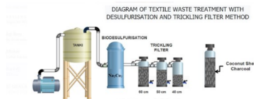
Picture of Bio Desulfurization Reactor and Trickling Filter
