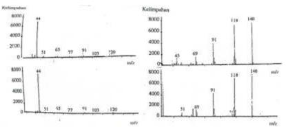
Figure 3. Standard mass spectrum of amphetamine and mass spectrum from gas chromatographymass spectrometry library
